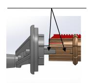
The disassembly and assembly of the lateral faces must be carried out very carefully because a bad tightening of the screw deteriorates the thread and the assembly becomes impossible.
