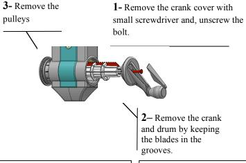
**4.2**– Regulation of the amount of scraped flakes **Left hand crank**
