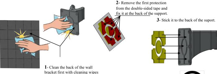
and then the wall. **4**- Remove the 2<sup>nd</sup> protection from double-sided tape
