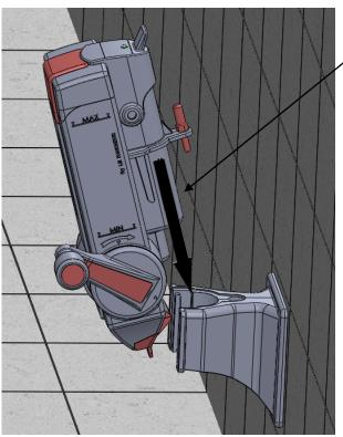
**6-** Slope the grinder 15 degrees before insert into the support.
