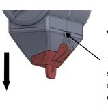
2- Clean the lower part and the nozzle of the grinder with a brush as well as the cutting blades.
