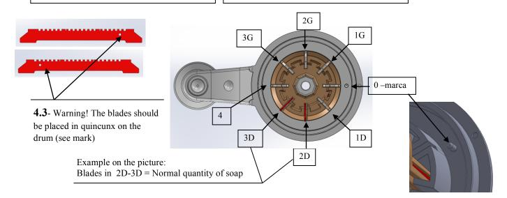
**5-** Replace the drum on the crankshaft carefully and by matching the groove with the fitting.
