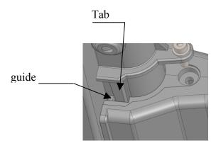
7- Sloped scraper to 15 degrees: insert into the soap grinder grooves and press firmly. Tighten the screw by hand or with a screwdriver (option).
